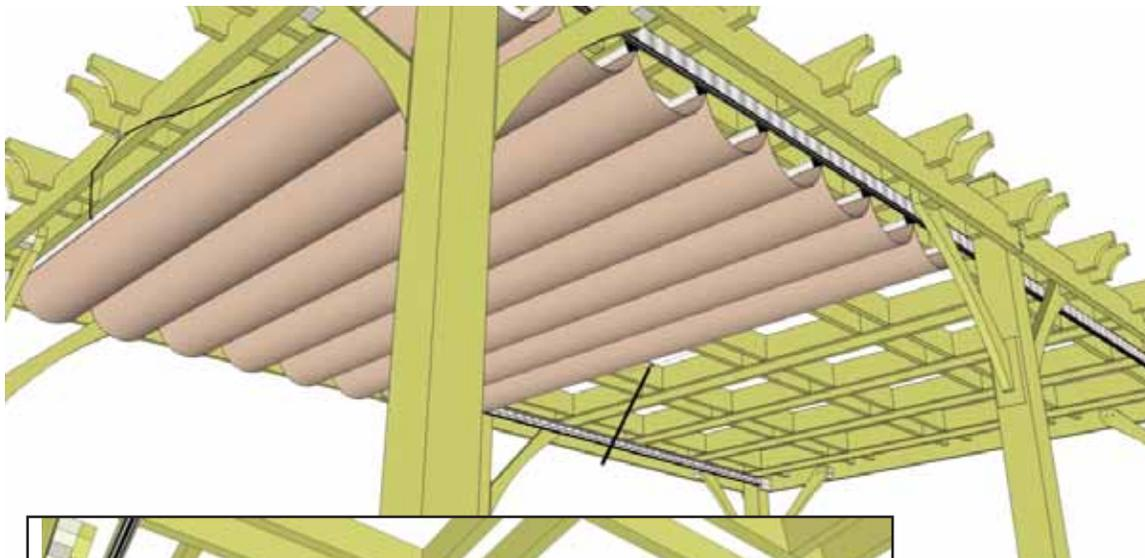
**14.** Extend and contract the canopy several times with pull handle. When extending or contracting the canopy, **pull** firmly in one continuous motion to prevent wings from binding.
