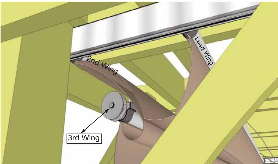
**9.** Continue to feed wings into the track until all wings are installed.
