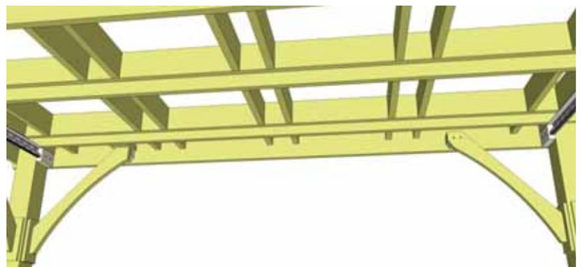
**10.** Install **Part D - 1 1/2" x 3 1/2" x 4 1/2" Wooden Wing Stops - 2 Pcs.** where track ends and gap exists. Use 2 - 2 1/2" brown screws per stop to install. When removing the wings and canopy in the future, simply remove wing stops on one end and roll wing and canopy out carefully with a helper.
