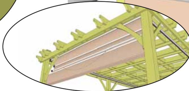
**8.** Push Lead Wing slightly ahead on track. Wings can roll out of track until **Part D - 1 1/2" x 3 1/2" x 5 1/2" Wooden Wing Stops** are installed so be careful. Lift and feed 2nd Wing into track and push wing slightly forward.
