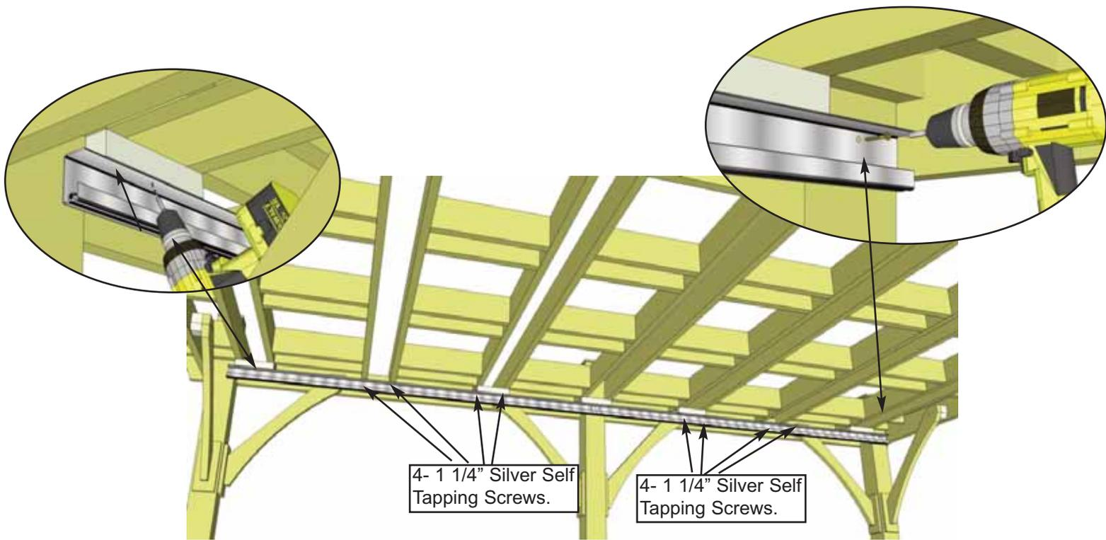
**5.** Align and attach second **Canopy Track** directly underneath lowering cleats as per Step 4. Position track with drilled end flush against post as illustrated above.
