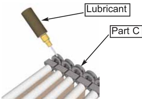
**6.** Prior to feeding **Part C - Aluminum Wings and Canopy** into track, locate Lubricant in Hardware Pack and apply a small amount to top of each wheel. Spin wheel slowly to lubricate entire surface. Complete all wheels.
