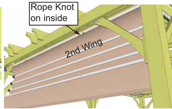
**7.** Before feeding **Part C - 133" long Aluminum Wings (9)** with **Canopy** into track, make sure canopy fabric is facing the correct direction. First, locate Lead and Anchor Wings in set. Both have a black pull rope attached. Make sure rope knots are facing to the inside and the pull rope is facing to the outside. Starting with the Lead Wing, feed the wing wheels onto the track as shown above. Wheels have springs and compress in and out slightly to fit.
