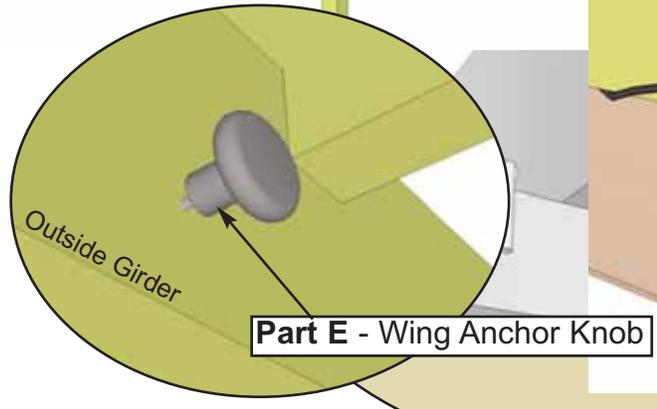
**12.** With canopy pull handle or on a ladder using your hand, pull anchor rope up tight so anchor canopy wing can't move. Confirm anchor wing wheel is against wooden wing stops. Center Anchor Knob from side-to-side and mark. Before attaching, make sure anchor rope will be snug when slipped over knob. Screw wing anchor knob into outside girder. Pre-drilling with 1/16" drill bit may be helpful.
