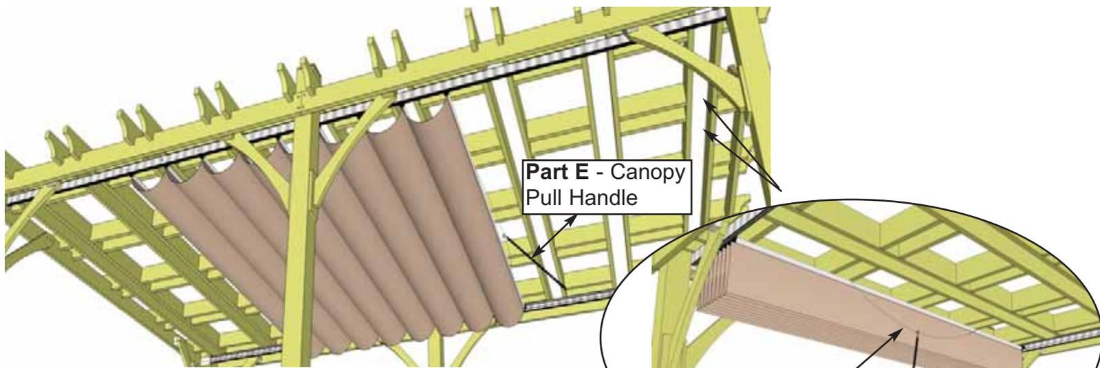
**11.** Using **Part F - Canopy Pull Handle**, pull canopy back and forth a few times to lubricate wheels and track. If wing binds, stop and pull forward until wings are straight and start again. When wings and canopy are tracking well, pull canopy to anchor side of pergola to install **Part E - Wing Anchor Knob**.
