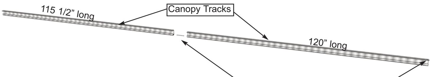
**2.** Locate **Part B's - 120" long (2 Pcs)** and **115 1/2" long Canopy Tracks (2 Pcs)** as well as **4" long x 1/4" diameter Plastic Track Connector (2 Pcs)**. Orientate track so counter sunk holes in long and short end of track are adjacent to each other. Push connector into track profile approximately 2" then push tracks together. Complete 2 sets of tracks.
